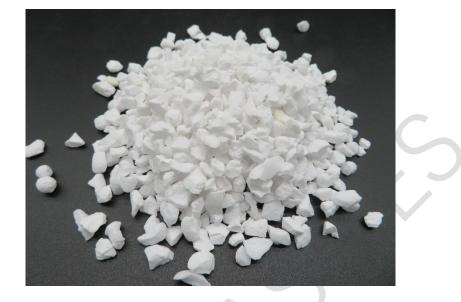
Tabular Alumina (TA) is a kind of  $\alpha$ -Al2O3 material which is rapidly sintered by high temperature shaft kiln then by rapid cooling. It has the characteristics of low open porosity and large crystals with closed spherical pores which are trapped upon re-crystallization during rapid sintering. Tabular alumina is of high refractoriness, excellent thermal shock resistant, fantastic anti-creeping and anti-stripping performance.
