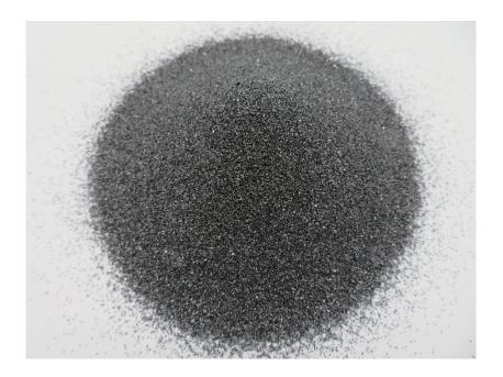
It is black and features brittle and sharp, certain capacity of heat-transmission and electricity-transmission. Its Knoop hardness is 3100-3280kg/mm². It can be used for making bonded and coated abrasives, which are suitable for grinding metal and non-metal materials with lower tensile strength, such as gray cast iron, brass, aluminium, stone, leather, rubber, paint, wood, etc. Besides, it can be also used for refractories.
